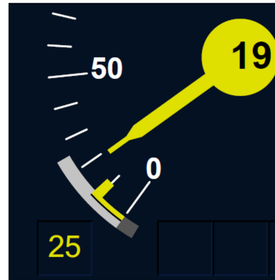
Figure 48 – Release speed, when V_{perm} < V_{relea}
