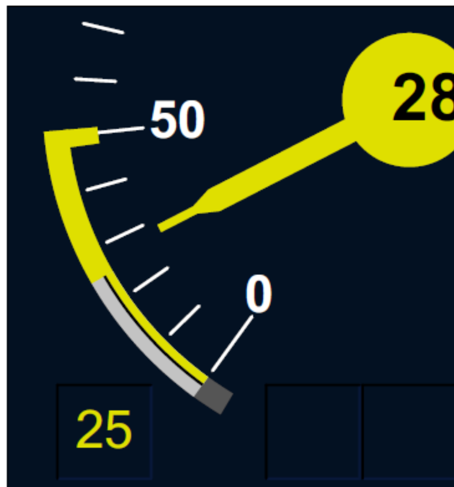
Figure 47 – Release speed, when V_{perm} > V_{relea}
